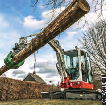
The new Takeuchi TB225 is a market first 2.5-tonne class mini excavator with expandable tracks, allowing it to become the new performance leader in towable mini excavators.
