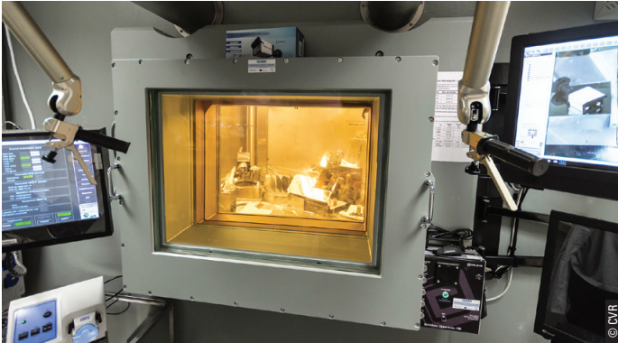
Hot cells in CVŘ meet new demands for material research of highly irradiated materials.
